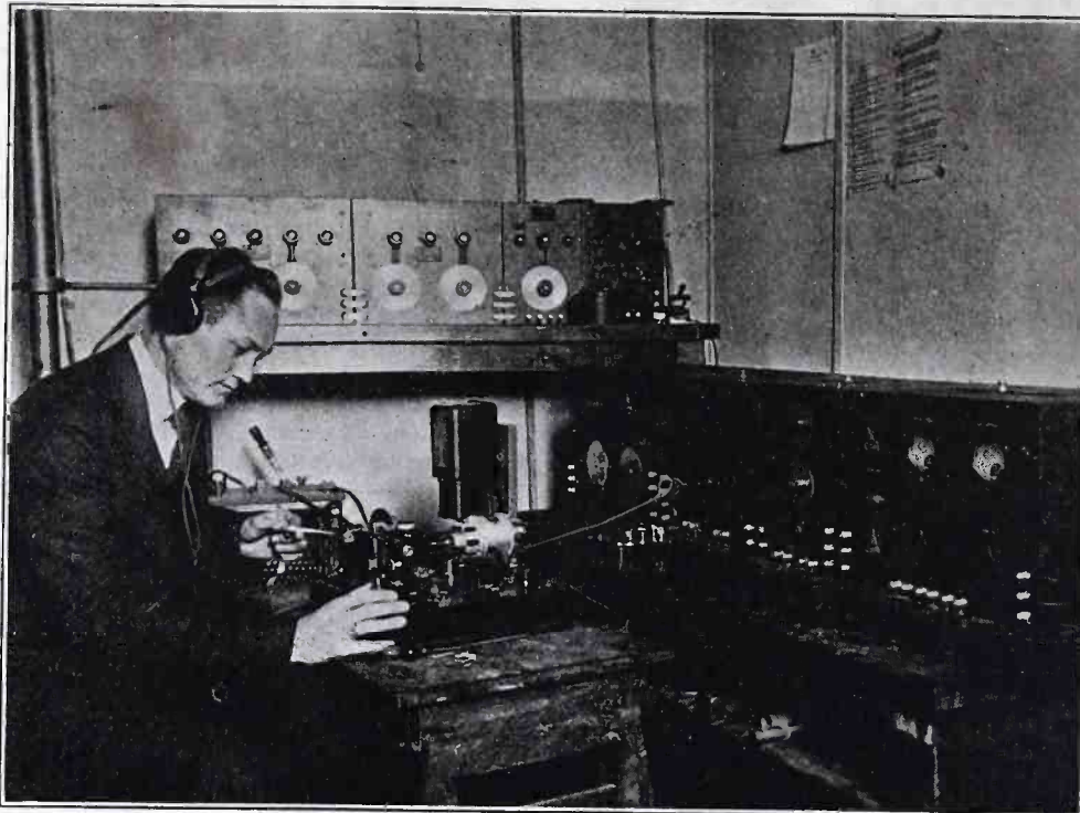
New Differential Recorder for Automatic Reception of Morse or Printing Telegraph Messages, As Devised by A. Hoyt Taylor, U. S. Navy Physicist
